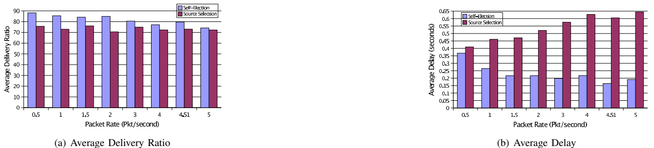
Fig. 16. Average Delivery Ratio and Average Delay comparison between two types of geographical forwarding, source selection using “hello” packets and receiver self-election using our RTS/CTS-based mechanism, under the scenario with obstacles. The routing protocol is RBVT-P, and the network size is 250 nodes.
