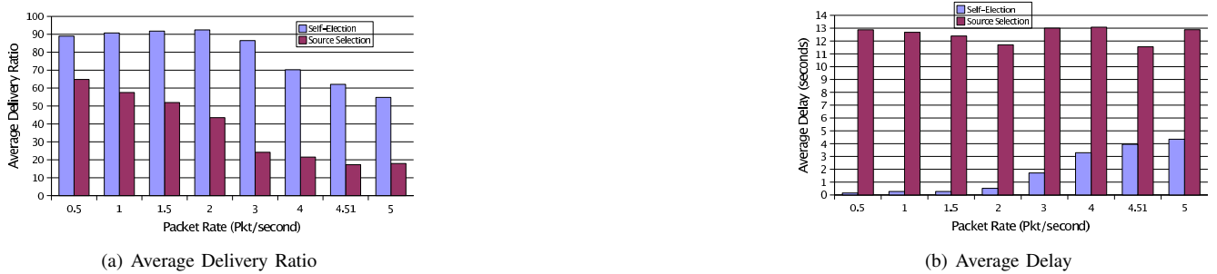
Fig. 15. Average Delivery Ratio and Average Delay comparison between two types of geographical forwarding, source selection using “hello” packets and receiver self-election using our RTS/CTS-based mechanism, under the scenario without obstacles. The routing protocol is RBVT-R, and the network size is 250 nodes.
