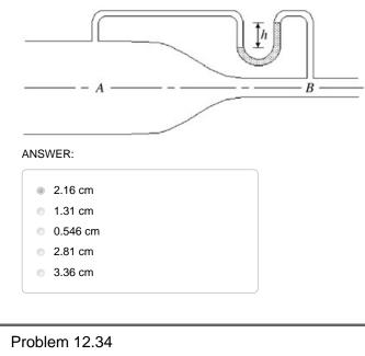
**Description:** (a) In a section of horizontal pipe with a diameter of 3.00 cm the pressure is 5.21 kPa and water is flowing with a speed of 1.50 m/s. The pipe narrows to 2.50 cm. What is the pressure in the narrower region if water behaves like an ideal fluid of...
