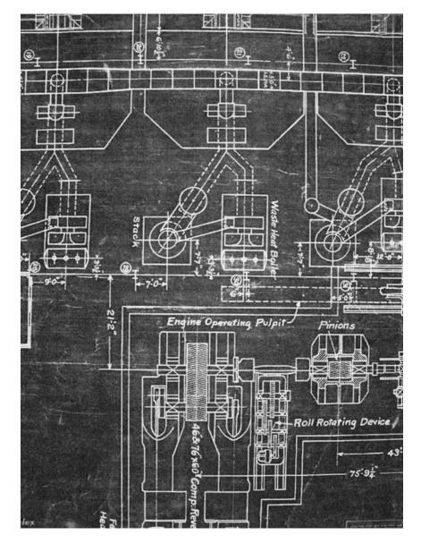
Figure 8. **Detail of the General Arrangement of the #5 Mill, Revised.** This is a small section from a blueprint floor plan, approximately three by five feet, that shows the placement and interaction of the machinery. This blueprint shows frequent use since it is ripped in half and additional revisions were made on fresh paper glued to the original.
