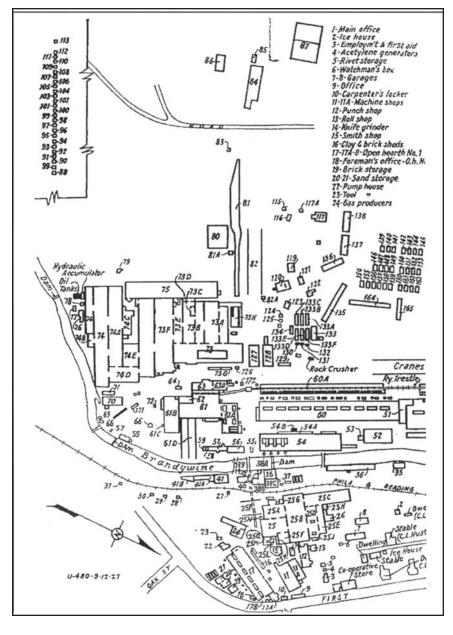
Figure 16. Ford, Bacon & Davis Map of Lukens Steel Company (1927). This map is adapted from a small blueprint image. It shows the size and complexity of the plant and identified each building on the site. The earliest portion of the plant is in the lower center.
