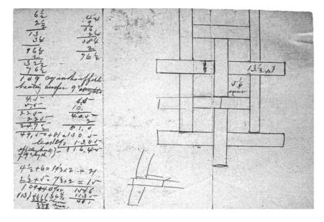
Figure 10. Sketch Used for Thought Processes. Charles Lukens Huston made these calculations to check the amount of exposed surface in the brickwork of the furnace structure proposed in the previous sketch (Figure 9).
