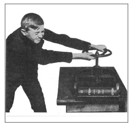
Figure 9. **Making a Letterpress Copy.** Each piece of correspondence, while the ink was still wet, was placed between two blotters and pressed onto a sheet of tissue paper [7, p. 26].
