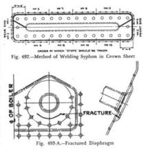
Figure 10. Page from Laying Out for Boiler Makers and Plate Fabricators. This is an example of a highly-specific technical manual containing both text and drawings [24].
