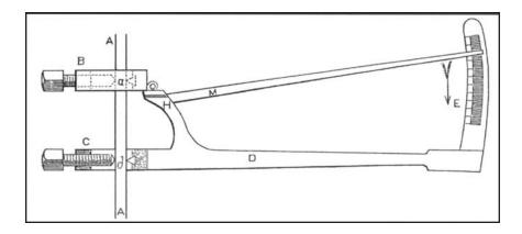
Figure 13. Dr. Charles Huston's Testing Apparatus (1879). Dr Huston designed this apparatus, later called an extensioneter, to test increasing strain on metal and described it in an article in the *Journal of the Franklin Institute*.
