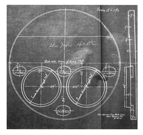
Figure 7. **Blueprint for Boiler Head, The Johnson Ironworks (1901).** This approximately three-foot by three-foot blueprint is one of many from customers specifying the product that they required. Blueprints were used for copying multiple images for engineering, building plans, and writing.
