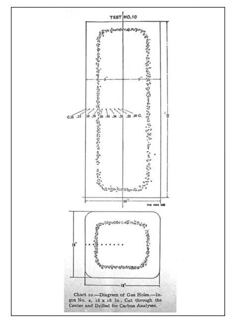
Figure 22. **Drawing Demonstrating Segregation of Steel in Ingot.** Also from Huston's article, this diagram shows the bubbles with the variation in carbon readings throughout the ingot.
