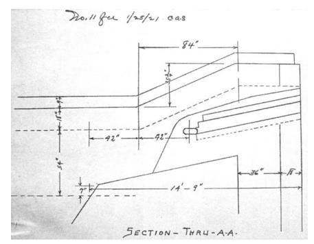
Figure 9. Sketch Used for Informal Communication (1921). The manager of operations sent this sketch to illustrate the planned changes in an open hearth furnace.
