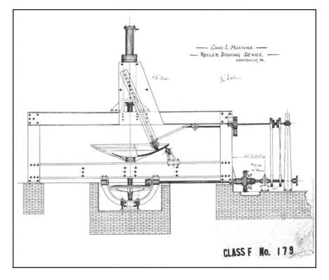
Figure 14. **Roller Dishing Device by Charles Lukens Huston.** This undated drawing was done on sized linen and is approximately three-feet by four-feet. It was probably drawn in connection with Huston's work on adding guides to an earlier device.
