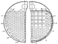
Fig. 490.-Method of Renewing Front Tube Sheet Area
