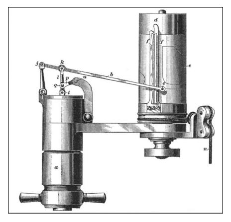
Figure 16. Indicator Card Device for Testing Engine Power. This device was attached to an engine to measure its power output. A card was attached to the drum and a pencil, connected to a pressure-measuring device, drew a diagram on the card [15].
