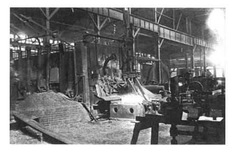
Figure 1. **Reheating Furnace.** Ingots or slabs of steel that did not go directly from the open hearth soaking pits to the rolls had to be heated in separate reheating furnaces.
