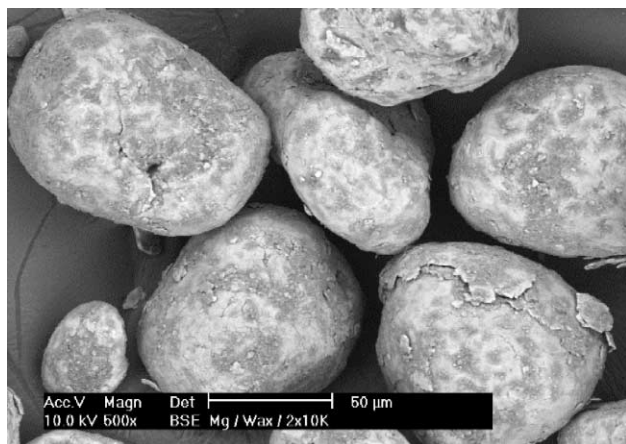
Fig. 27. Surface morphology of magnesium particles coated in the hybridizer for 2 min at 10,000 rpm with 2% wax.
