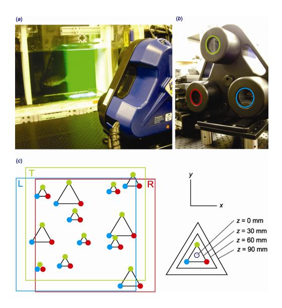
**Figure S1.** (a) Camera probe relative to bluegill swimming in front of laser volume in flow tank. (b) Front view of the camera probe. (c) Illustration of particle triangulation technique; modified from Troolin and Longmire (2010).
