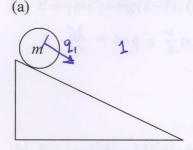
A disk rolling without slipping down a fixed incline
