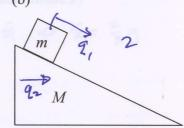
A block sliding without friction down an incline that is also free to slide without friction.
