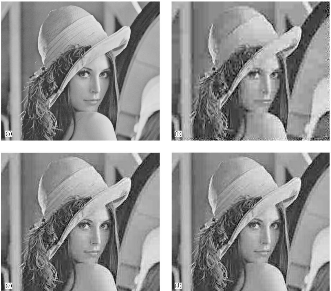
Fig. 7. (a) Part of original Lena image (size 446 \times 510 ); (b)–(d) reconstructed Lena images with 2M = 16 , bit rate 0.1 bpp, and ELT prototype; (b) image size 446 \times 510 , insertion at the end of rows and columns with the modified subband values y'_6(c) = y''_M(c - 1) = 0 , PSNR = 25 dB; (c) image size 446 \times 510 samples, modified subband values y'_6(c) = y''_3(c - 1) = 0 , PSNR = 29 dB; (d) image size 448 \times 512 , PSNR = 29.2 dB.
