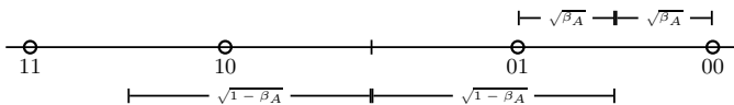
Fig. 3. The superposition modulation employed at Node A. Node B adopts a similar modulation with a possibly different superposition factor \beta_B . The left bit in the label is the local bit, while the right bit is the relay bit.
