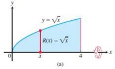
This method for calculating the volume of a solid of revolution is often called the **disk** method because a cross-section is a circular disk of radius R(x).
