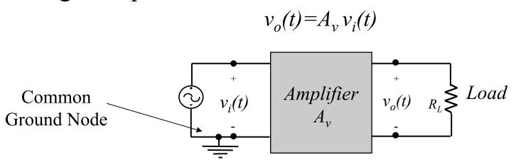
•  $A_v$  is called the voltage gain and if <0 then the amplifier is inverting; otherwise non-inverting.
