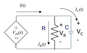
We could have gotten this from calculating the impedance. Since R and C are in parallel we have using the reciprocal rule:
