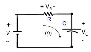
*Note*: In general the time constant is equal the total resistance which is in series with the total capacitance.
