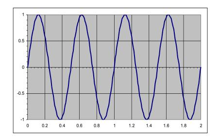
As stated previously, increasing the **Timebase** further will display more cycles. However, to display one cycle of the 2 Hz sine wave, the **Timebase** needs to be reduced to 50 milliseconds/division (since the inverse of the frequency 2 Hz = 0.5 seconds is the signal's period and since our scope has 10 divisions, we have 50 milliseconds).
