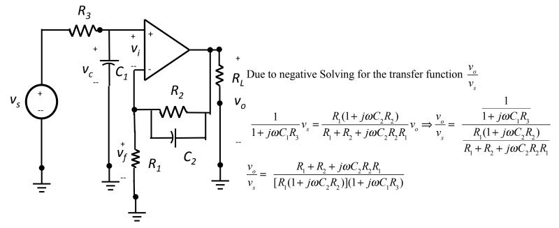
$$\frac{v_o}{v_s} = \frac{R_1 + R_2 + j\omega C_2 R_2 R_1}{[R_1(1 + j\omega C_2 R_2)](1 + j\omega C_1 R_3)} = \frac{R_1 + R_2(1 + j\omega \frac{C_2 R_2 R_1}{R_1 + R_2})}{R_1[1 - \omega^2 C_2 R_2 C_1 R_3 + j\omega (C_1 R_3 + C_2 R_2)]}$$
