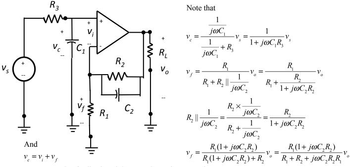
Due to negative feedback and the summing point constraint
