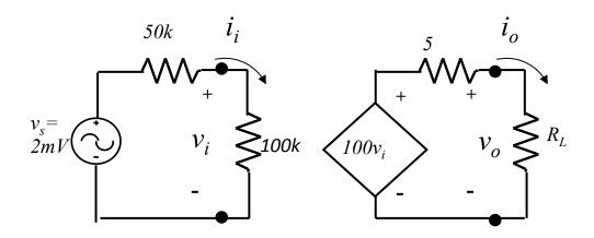
1. For the following circuit, determine the value of  $R_L$  to maximize the power gain for this circuit. Provide a proof. Which value of  $R_L$  makes the better design and why?
