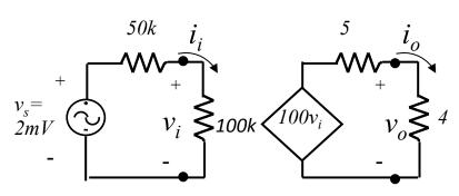
$$\frac{dG}{dR_L} = \frac{1}{(R_L + r_o)^2} r_i A^2 - 2 \frac{R_L}{(R_L + r_o)^3} r_i A^2 = 0$$
