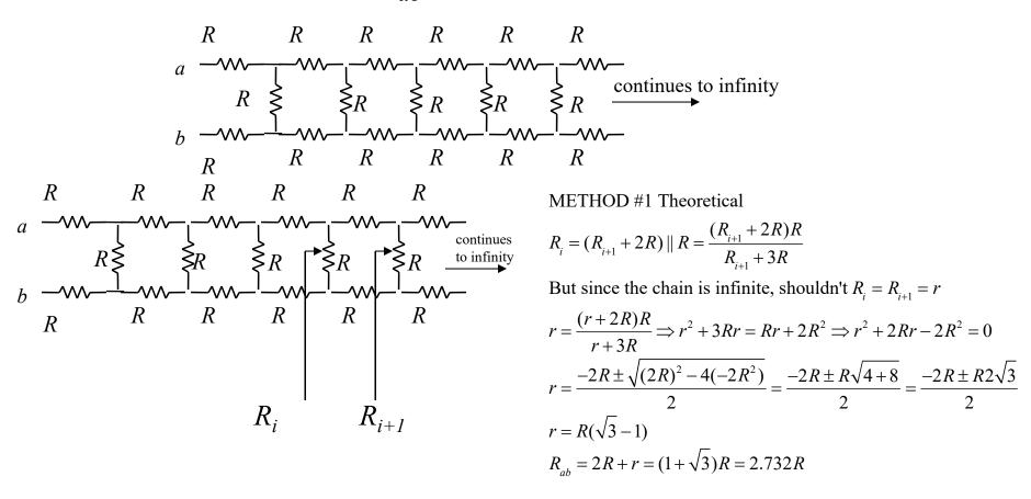
Find the total resistance  $R_{ab}$  for this infinite resistive network
