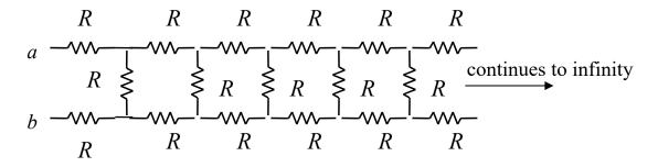
Find the total resistance  $R_{ab}$  for this infinite resistive network
