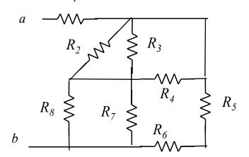
In this circuit R5 and R6 are in series. In addition, R4, R3, and R2 are in parallel. Finally R7 and R8 are in parallel. These two parallel combinations are in series. This series combination is in series with the series combination of R5 and R6. R1 is in series with this parallel combinations. This is
