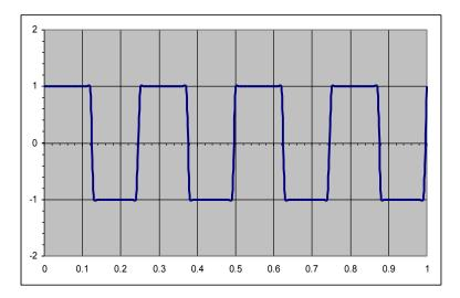
Therefore, knowing the approximate maximum frequency of the input signal is the guiding factor for choosing an appropriate value for the **Timebase**. Recall that the inverse of the maximum frequency of a periodic signal will yield the (time) **period** of 1 cycle. Therefore, the **Timebase** should be calculated by taking the **period** of the signal and dividing it by the number of horizontal X-axis divisions times the desired number of cycles to be displayed.
