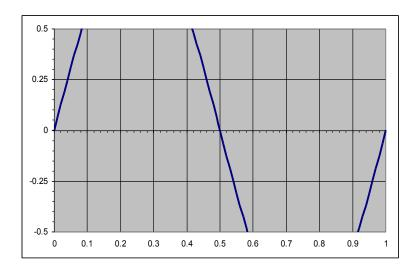
Likewise, setting it too high, and you'll won't find the signal. This figure shows the same sine wave with a **Volts/Div** of 50 volts/division.
