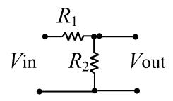
$$Vin = IR_{1} + IR_{2} = I(R_{1} + R_{2})$$
