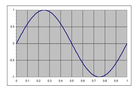
Setting the **Timebase** to 200 milliseconds/division X 10 divisions = 2 seconds will yield a display of 2 cycles.
