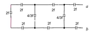
$$CA = 2 \text{ in series } 2 \text{ in series } 2 = \frac{1}{\frac{1}{2} + \frac{1}{2} + \frac{1}{2}} = \frac{2}{3}$$
