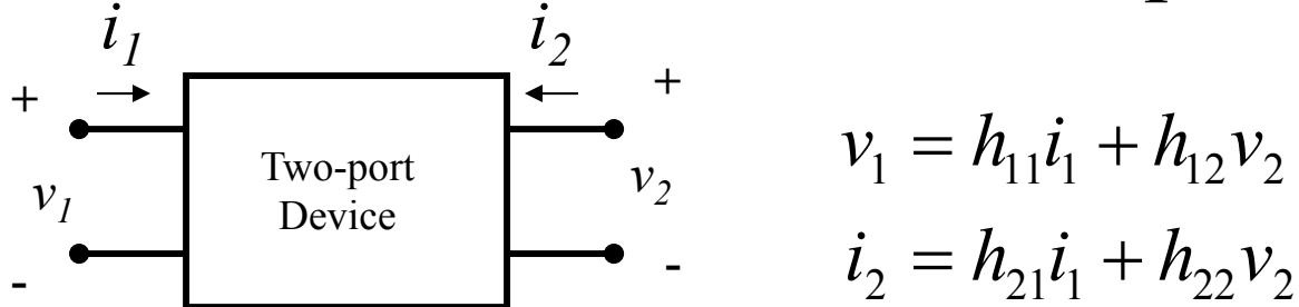
11  $\Rightarrow$  input relationship;  $h_{11} = \left. \frac{v_1}{i_1} \right|_{v_2=0}$  = input resistance with output shorted-circuited
