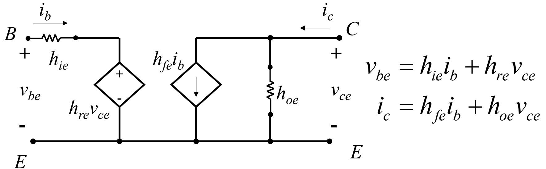
The parameters defined by this equivalent circuit as usually provided by transistor manufacturers to describe the performance of the BJT. For example,  $\beta$  and  $h_{fe}$  are typically given in BJT data sheets.
