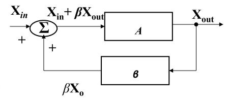
Practically, we make  $\beta(f)A(f)$  slightly > 1 ( $\mathbf{X}_{out}$  grows) at the frequency of oscillation. (Otherwise, the signal will decay to zero.) This causes clipping eventually but ultimately, a constant amplitude results. (This method enables some wave shaping to yield waveforms other than a sinusoid.)
