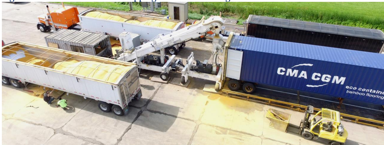
Figure 2: Containerized Grain Shipping with Transloading
