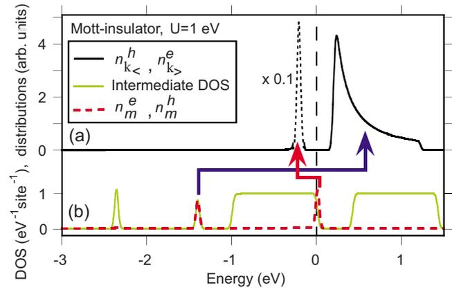
FIG. 6. (Color online) (a) Occupation of holes and electrons for the Mott insulator with  $U=1$  eV similar to the one shown in Fig. 4(b). For illustrative purpose, a smaller core-hole potential ( $U_c = 2$  eV) is chosen. (b) Intermediate DOS shown in gray (green) solid line and  $n_m^e$  and  $n_m^h$ , defined in the text, in (red) dashed line. Arrows indicate how the two plots are related, as explained in the text.
