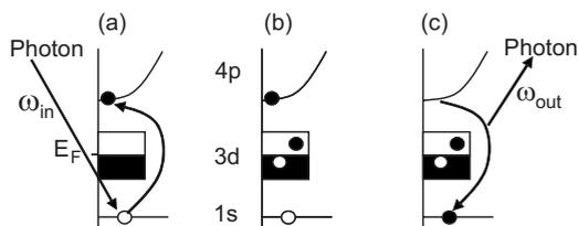
FIG. 1. Illustration of the RIXS process studied in our work, that is, transition-metal oxide *K*-edge RIXS. This process is distinguished from other types of RIXS, such as transition metal oxide *L*-edge RIXS (Figs. 1 and 2 in Ref. 11), *K*-edge RIXS for diamond or graphite (Fig. 3 in Ref. 12), or *K*-pre-edge RIXS for cuprates (Refs. 13 and 14).
