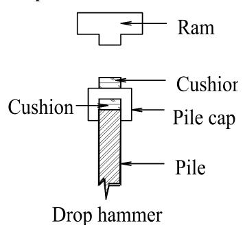
$<sup>^1</sup>$  Very noisy, simple to operate and maintain, 5-10 blows / minute, slow driving, very large drop, not suited for end bearing piles, used on Franki piles
