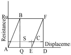
Q - displacement called quake where resistance reaches Ru
