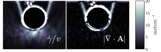
FIG. 3. The local shear rate  $\dot{\gamma}/v$  and the divergence of  $\mathbf{A}$ , computed numerically from the flow field shown in Fig. 2(a), showing that  $\mathbf{A}$  is a divergence-free shear flow.
