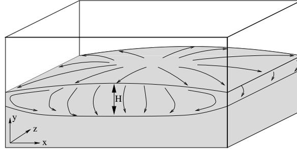
Fig. 2. – Sketch of time-averaged convection flow lines in the liquefied layer. Magnitude of the flow in  $y$  and  $z$  directions has been greatly exaggerated.
