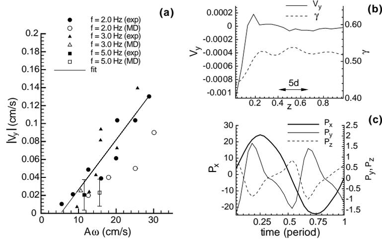
Fig. 4. – (a) The average speed at which grains fall along the shearing wall *vs.* shearing speed  $A\omega$  of the wall; the line is the least square fit to experimental data. The error bars show two typical standard deviations. (b) MD results for  $v_y$  (in units of  $A\omega$ ), and for solids fraction  $\gamma$  ( $A = 1$  cm,  $f = 2$  Hz). The diameter of the particles,  $d = 2$  mm, is also shown. (c) Total momentum (in arbitrary units) during one period (MD).
