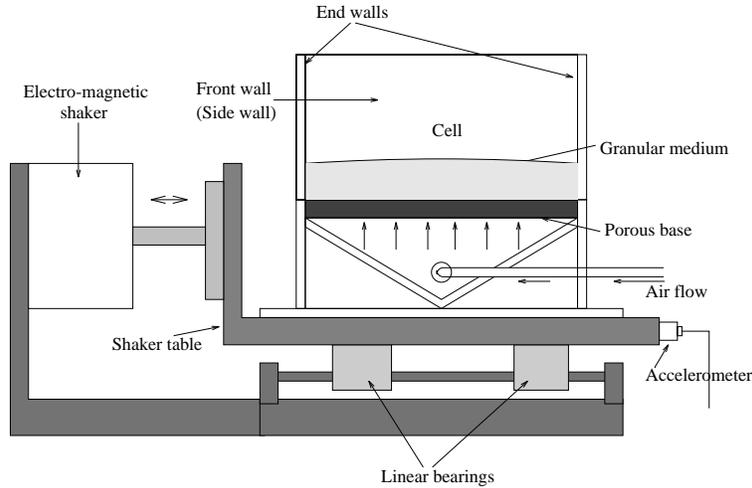
Fig. 1. – Schematic of the apparatus. The cell is made of Plexiglas, and is mounted on a Plexiglas base of the same cross-sectional dimensions which is attached to a table. An electro-mechanical actuator, driven by a sinusoidal AC signal, provides the horizontal driving.
