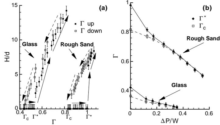
Fig. 3. – (a) Thickness of the liquefied layer next to the side walls ( $x$ - $y$  plane) vs.  $\Gamma$  for glass beads,  $d = 0.6$  mm and rough sand  $d_{\text{ave}} = 0.6$  mm.  $\Gamma^*$  and  $\Gamma_c$  are the bifurcation points when  $\Gamma$  is increased and decreased quasi-statically. (b) Bifurcation points  $\Gamma^*$  and  $\Gamma_c$  vs. dimensionless lifting pressure.
