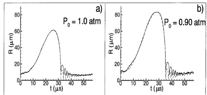
FIG. 3. The experimental results (broken lines) and the fits (solid lines) for two values of ambient pressure,  $P_0$ . In (a) the acoustic pressure amplitude,  $P_a$ , and  $R_0$  are used as fitting parameters ( $R_0 = 7.3 \mu\text{m}$ ,  $P_a = 1.29 \text{ atm}$ ); in (b) we use  $P_a = 1.29 \text{ atm}$ , and fit only  $R_0 = 9.0 \mu\text{m}$ . The liquid viscosity is  $0.021 \text{ cm}^2/\text{s}$ , and surface tension is  $69.4 \text{ dyn/cm}$ .
