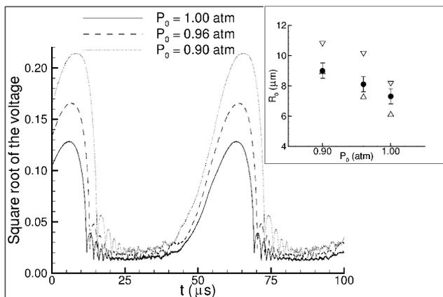
FIG. 2. Experimental  $R(t)$  curves as ambient pressure  $P_0$  is varied. The inset shows the results for  $R_0$ : experiment ( $\bullet$ ), and diffusion theory ( $\Delta$  and  $\nabla$ ) obtained assuming polytropic exponent  $\gamma = 1.0$  and  $1.67$ , respectively. The estimated combined experimental and fitting uncertainty is also shown.
