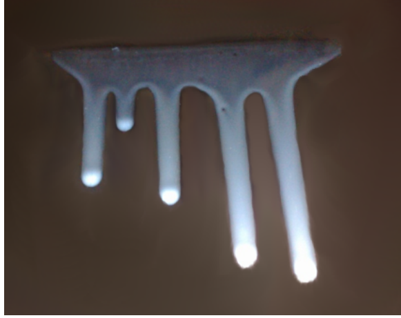
Figure 9: Image of line of NLC flowing down silicon wafer.
