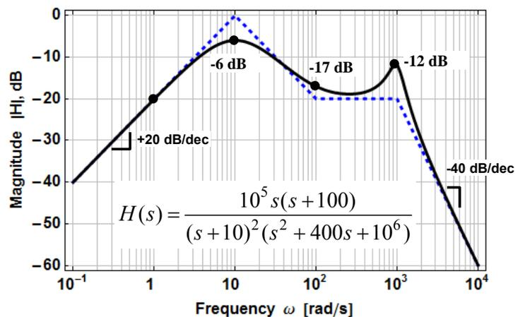
Figure 1-12 – Example problem integrating many common features of Bode plots.
