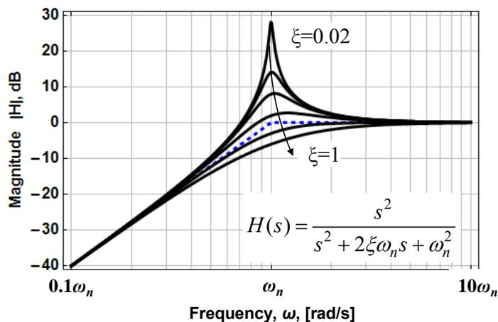
Figure 1-11 – Amplitude response for the general 2<sup>nd</sup>-order high-pass function for various values of  $\xi$ .
