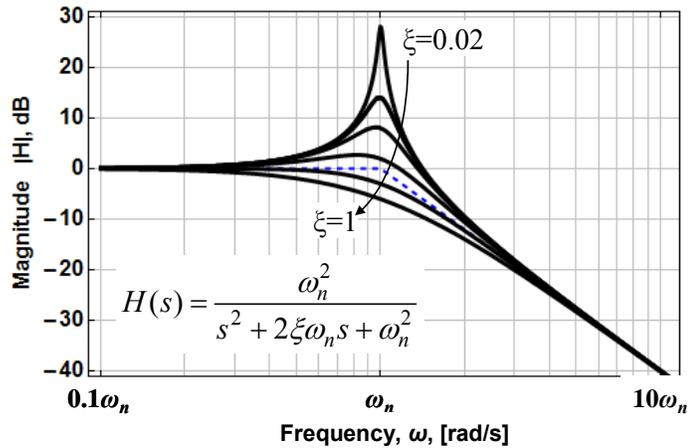
Figure 1-8 – Bode amplitude plot for the general 2<sup>nd</sup>-order low-pass response for various values of  $\zeta$ .
