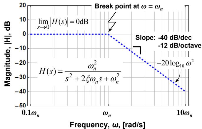
Figure 1-7 – Uncorrected Bode amplitude plot for a second-order response with  $0 \leq \xi \leq 1$ .
