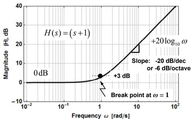
Figure 1-2 – Frequency response for a simple zero at  $s = -1$
