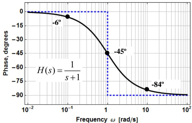
Figure 1-14 – Bode phase plot for a simple pole at  $s = -1$
