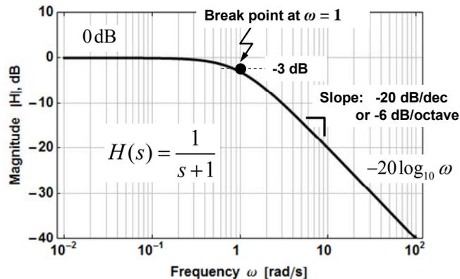
Figure 1-1 – Frequency response for a simple pole at  $s = -1$
