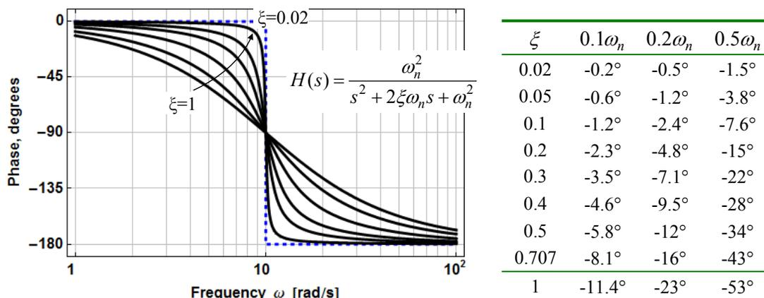
Figure 1-19 – Phase plot for a 2<sup>nd</sup>-order low-pass response as a function of the damping factor. Numerical data at three frequencies below the break are tabulated as an aid for sketching the response.
