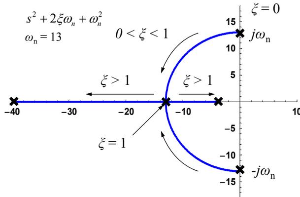
Figure 1-13 – Root-locus in the complex plan for the second-order polynomial as a function of damping factor.
