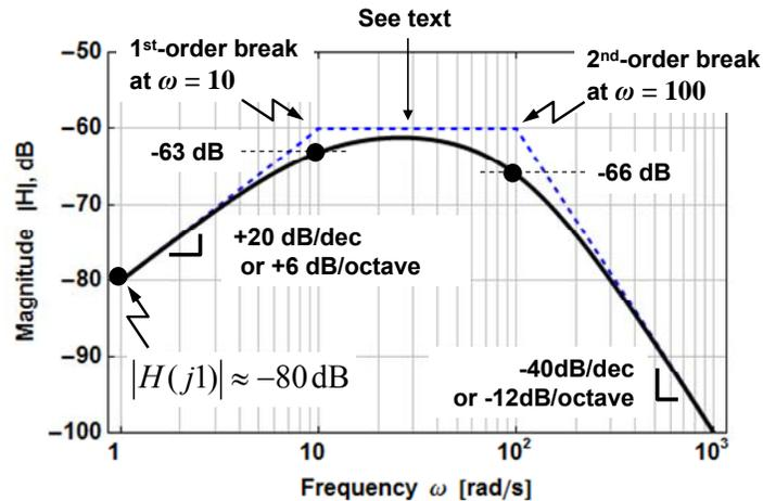
Figure 1-6 – Bode plot for the function given in (1.24)
