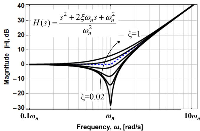
Figure 1-10 – Amplitude response with a complex zero pair.
