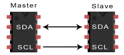
So far, we've talked about the basics of <u>SPI communication</u> and <u>UART</u> <u>communication</u>, so now let's go into the final protocol of this series, the Inter-Integrated Circuit, or I2C.
