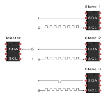
6. To stop the data transmission, the master sends a stop condition to the slave by switching SCL high before switching SDA high:
