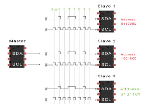
3. Each slave compares the address sent from the master to its own address. If the address matches, the slave returns an ACK bit by pulling the SDA line low for one bit. If the address from the master does not match the slave's own address, the slave leaves the SDA line high.
