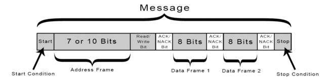
**Start Condition:** The SDA line switches from a high voltage level to a low voltage level *before* the SCL line switches from high to low.
