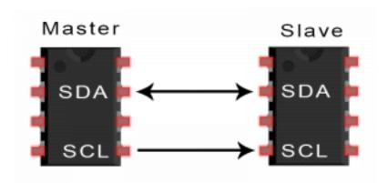
SDA (Serial Data) - The line for the master and slave to send and receive data.
