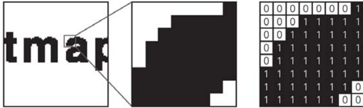
Figure 1.2. An enlargement of a monitor's display of the word tmap and the corresponding bits for each pixel.
