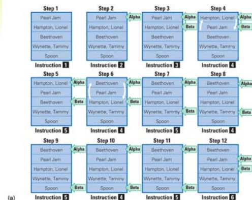
Figure 10.2. The steps of Alphabetize CDs algorithm. A snapshot of the CD rack is shown at the completion of each instruction. Notice how Beta sweeps through all of the slots following Alpha. After the first 11 steps, the alphabetically earliest CD, Beethoven, is in the Alpha slot.
