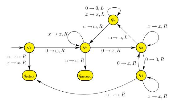
In each of the parts below, give the sequence of configurations that M enters when started on the indicated input string.
