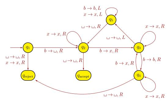
4. **[10 points]** The Turing machine M below has input alphabet  $\Sigma = \{b\}$  and tape alphabet  $\Gamma = \{b, x, \sqcup\}$ .
