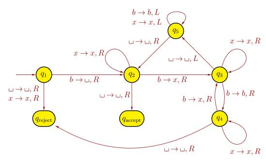
3. **[10 points]** The Turing machine M below has input alphabet  $\Sigma = \{b\}$  and tape alphabet  $\Gamma = \{b, x, \sqcup\}$ .
