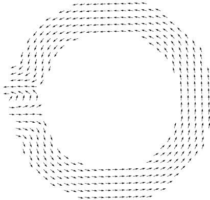
Fig. 2. Bit-encoding magnetization state with a  $-360^\circ$  wall on the left. The other bit is encoded by the mirror image of this magnetization pattern, with the  $+360^\circ$  wall on the right, respectively. From the numerical solution of (3), see the text for details.
