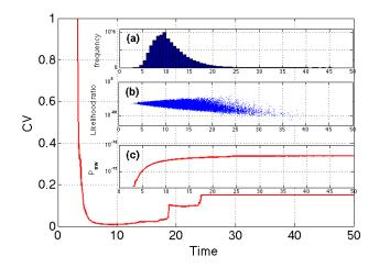
Fig. 3. CVs of IS estimators for  $I_J = 0.3$  with infinite-time bias functions and sample size  $10^5$ . Inset (a) is a histogram of exit times for the biased system. Inset (b) is the estimated likelihood ratio vs. time. Inset (c) is the probability of switching before time *T*. The sample size here is  $M = 10^5$ .
