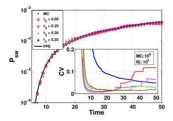
Fig. 4. Switching probabilities and CVs of IS estimators for  $I_J = 0.6$  with infinite-time bias functions active outside of a region containing the stable fixed point, defined by  $\theta_0 < |\theta| < \theta_J$ , for different values of  $\theta_0$ . The sample size is  $10^5$ .
