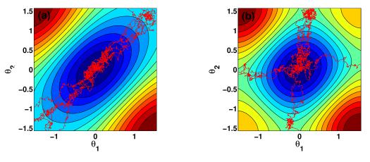
Fig. 7. Sample paths from IS for two-spin systems with current  $I_J = 0.1$  and thermal stability factor  $\Delta = 60$ : (a) strongly coupled spins with c = 0.8 and (b) weakly coupled spins with c = 0.2. False color corresponds to the effective potential in (23).
