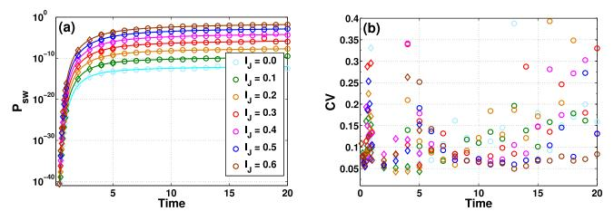
Fig. 2. Similar to Fig. 1, but with  $\Delta = 30$ . For  $T \ge 4$ , infinite-time bias functions are used, and for  $T \le 5$ , finite-time bias functions are used. IS estimates at T = 4 and T = 5 obtained using infinite- and finite-time bias functions are indistinguishable. (a) RSER versus reading pulse duration T. (b) CV of the RSER.
