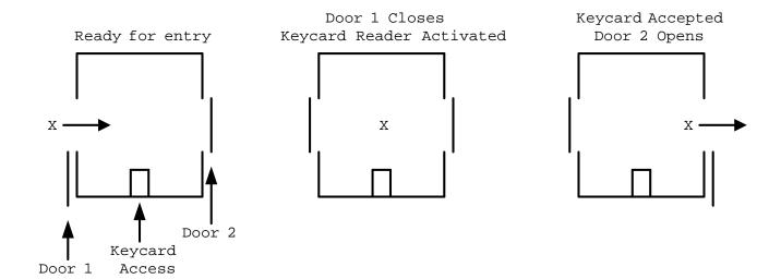
A mantrap is a physical access control that requires one person at a time enter through a door. Also known as air locks, sally ports, or access control vestibules, mantraps are used to prevent tailgating, or following another person through a secured door. These devices are often used with keycards to ensure that only people who are supposed to have access to a building can get in.
