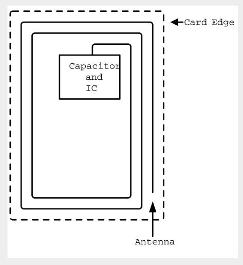
around the outside. This antenna is designed to be resonant at 125 kHz and when powered by the field created by the reader it charges a capacitor and provides current to an IC. The IC then broadcasts the card's ID.
