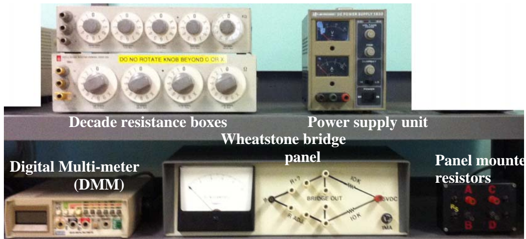
Figure 2 Experimental set up for Wheatstone bridge lab.
