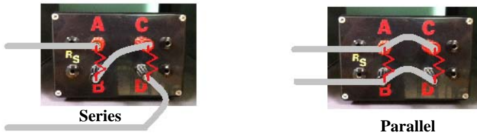
Figure 3 Panel mounted resistors AB and CD, when connected in series and parallel
