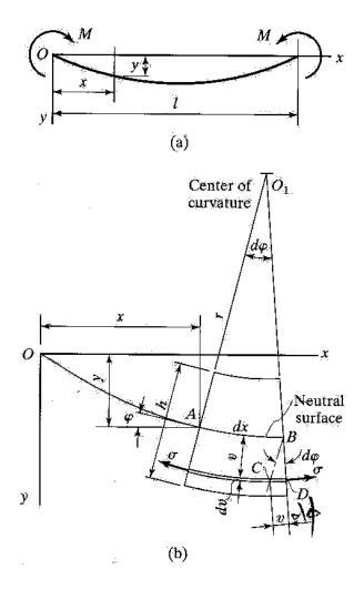
Slope of the beam at  $x = \phi$ ,  $\mathbf{f} = \frac{dy}{dx} & \frac{d\mathbf{f}}{dx} = \frac{d^2 y}{dx^2}$   $\frac{d\mathbf{f}}{dx} = -\frac{1}{r} = \frac{d^2 y}{dx^2}$   $\frac{d^2 y}{dx^2} = -\frac{M}{EI}$ fundamental beam equation
