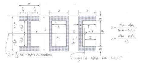
NA passes through the **Center of gravity** (**CG**) of the beam cross section. For rectangular or circular crosssection of the beam, CG is at the geometric center of the section.
