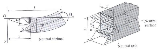
Let dA is an elemental area at a distance v from the neutral plane. The force acting on the element dA is the area multiplied by the bending stress, i.e.  $\sigma * dA = EvdA/r$ . The total force can be obtained by integration of all forces acting on the face.
