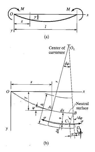
We can determine the bending strain and stress from the geometry of bending.
