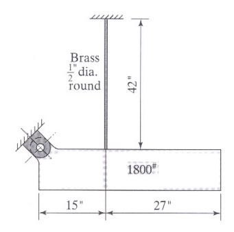
3. In the lower member is of uniform cross section and can be assumed to be rigid. Find the change in elevation of the left end because of the stretch of the rods.
