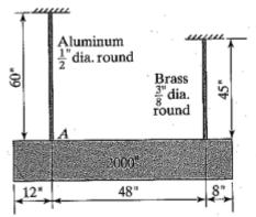
4. The members in the figure below have a neat fit at the time of assembly. Find the force caused by an increase in the temperature of  $50^{\circ}$ C. Supports are immovable.
