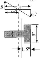
5. The inclined load shown in view M—M, Fig. 1-91, is applied to the pin at the end of the beam. Resolve load into horizontal and vertical components and find the bending stress due to each. Add algebraically to get stress at points A, B, C, and D. Ans. At A, σ = 1562.5 psi.
