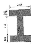
4 Find the values and plot the distribution of stress over the cross section of the upright Locate the point of zero stress.
