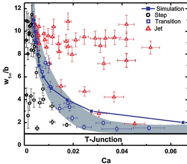
**Fig. 4** Phase diagram demonstrating the transition of jet-regime (red triangles) to step-regime (black circles). Blue open squares denote the transition regime, where droplet production alternates between step- and jet-regime. Blue solid squares indicate the simulation results for  $A = 0.4$ , as discussed in the text. For  $w_{1\infty}/b \leq 1$ , no stable filament is formed (color figure online)
