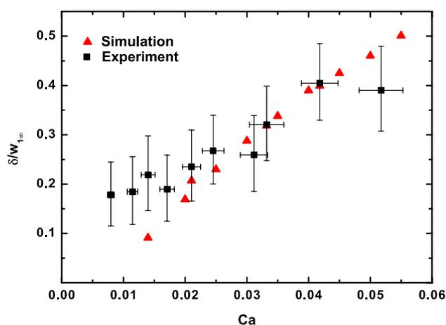
**Fig. 6** Comparison of the experimentally determined shape factor,  $\delta/w_{1\infty}$ , for  $Q_{1\infty}/Q_{2\infty} = 3$  (black squares) and the simulation results (red triangles) for  $Q_{1\infty}/Q_{2\infty} = 2.81$  and  $A = 1$  (color figure online)
