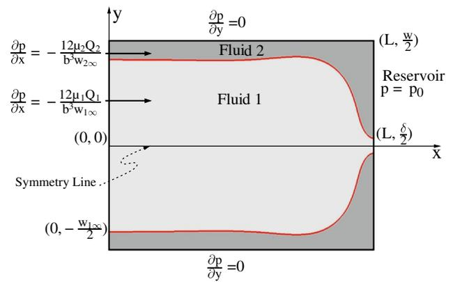
**Fig. 2** Schematic of the flow domain for the Hele-Shaw model and the corresponding boundary conditions. The domain is bounded by walls at  $|y| = w/2$ . At  $x = 0$ , fluid 1 occupies  $|y| \leq w_{1\infty}/2$  and fluid 2 occupies  $w_{1\infty}/2 < y \leq w$  and  $-w < y < -w_{1\infty}/2$ ;  $w_{2\infty} = w - w_{1\infty}$
