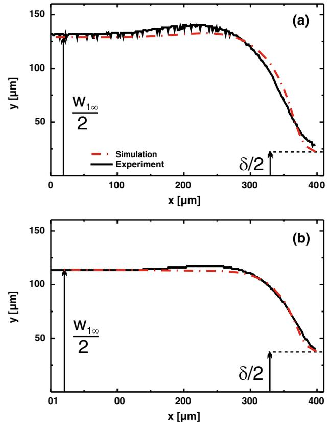
**Fig. 5** Comparison of the tongue profiles in the terrace obtained from experiments (black solid line) and simulations with  $A = 1$  (red dashed line). Both experimental profiles are obtained in the jet-regime. **a**  $Ca = 0.019$  and  $w_{1\infty}/b = 7.97$  and **b**  $Ca = 0.042$  and  $w_{1\infty}/b = 7.44$ . For experiments,  $Q_{1\infty}/Q_{2\infty} = 1.5$ . For simulations,  $Q_{1\infty}/Q_{2\infty} = 1.67$  in (a) and  $Q_{1\infty}/Q_{2\infty} = 1.41$  in (b) (color figure online)
