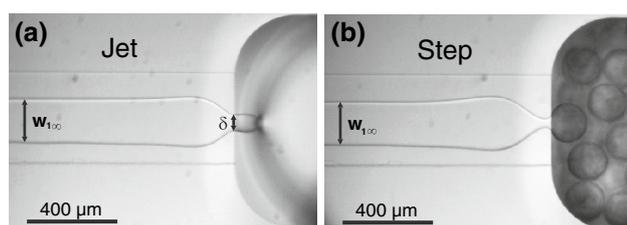
**Fig. 1** Optical micrographs showing two regimes of droplet production. **a** “Jet-emulsification” for large  $Ca$ : breakup occurs downstream, **b** “Step-emulsification” for low  $Ca$ : breakup occurs at the step
