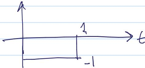
$$\begin{aligned} a. \quad E_0 &= \int_0^1 (1-2t)^2 dt = \int_0^1 (1+4t^2-4t) dt = \left[ 1 + \frac{4t^3}{3} - 4\frac{t^2}{2} \right]_0^1 \\ &= 1 + \frac{4}{3} - 2 = \frac{1}{3} \end{aligned}$$
