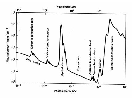
Hypothetical absorption spectrum for a typical III-V semiconductor as a function of phonon energy.
