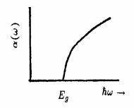
Frequency dependence of the absorption coefficient near a threshold for interband transitions.
