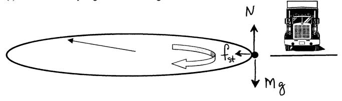
(b) What is the minimum radius R of the curve for which the truck can round the level curve without skidding?
