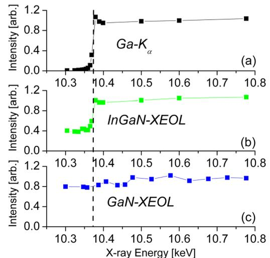
FIG. 3. (a) (Color online) Ga- $K\alpha$  fluorescence yield, (b) InGaN MQW x-ray excited optical luminescence (XEOL) yield, (c) GaN XEOL yield. All measured from the *c*-planar grown InGaN/GaN MQW sample.
