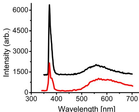
FIG. 1. (Color online) XEOL spectra for both *c*-planar (top/black curve) and *m*-planar (bottom/red curve) grown GaN/InGaN structures. The strong peaks at 365 nm originate from the GaN substrate; while the broad peaks at  $\sim 560$  nm originate from the InGaN/GaN MQW structures. Spectra were offset for clarity. These measurements were carried out at the Advanced Photon Source (APS) at Argonne National Laboratory.
