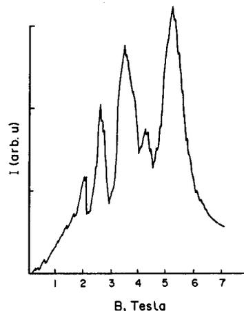
Fig.2. Magnetic oscillations of the total intensity at the Raman shift of the FA<sub>-1</sub> mode at  $T=30K$ .
