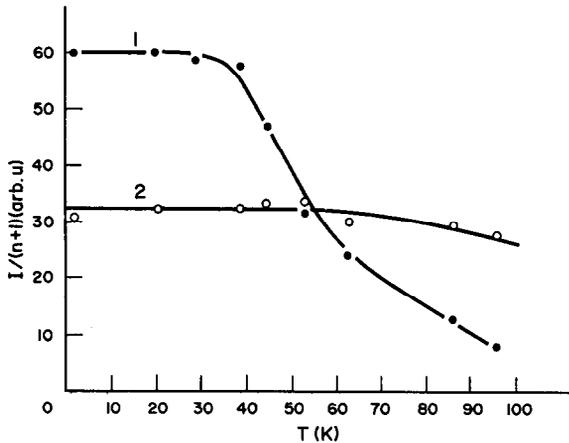
Fig. 3. Temperature dependence of the reduced intensity (I divided by the Bose factor) of the background (1) and the FA-phonon (2) at the Raman shift of the FA<sub>-1</sub> mode.
