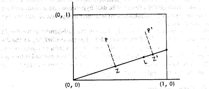
**Fig. 4.** Adjustment of absolute probabilities by computing the nearest point on the line defined by the cross-impact matrix.
