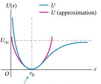
When r is near  $r_0$ , the potential-energy curve is approximately parabolic (as shown by the red curve) and the system behaves approximately like a harmonic oscillator.
