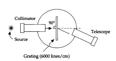
8. The angle at which the telescope must be located to observe the second order image of light of wavelength 589.3 nm is approximately
